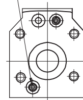
Pipe plug Removed for internal drain
